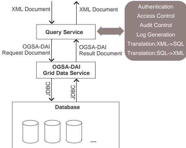
Figure 2: Grid Query Service Architecture
