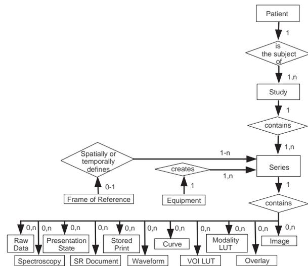
Figure 1: DICOM Entity Relationship Diagram
